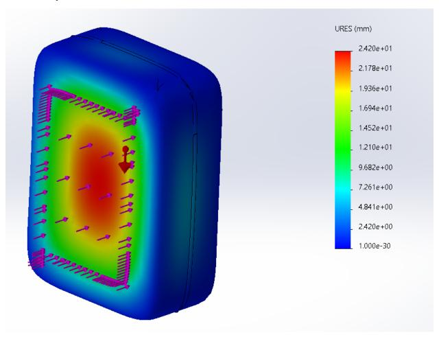
The stress analysis shows that the displacement of the luggage ranges from almost 0 to 2.420e+01 mm, decreasing gradually from the center of the area where the force is applied to the edge of the suitcase. There is also some deformation on the sides of the suitcase, at around 7.261 mm. Given that the length from front to back of the suitcase is 200 mm, this is an acceptable rate of deformation, as the suitcase could be further reinforced by personal items put inside during travel.
