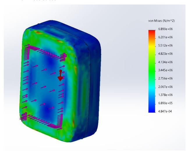
The stress analysis shows that the von Mises stress placed on the luggage ranges from 4.847e-04 to 6.890e+06 N/m², with 3.445e+06 N/m² being the most common value. The stress zone is primarily located around the area between the area where the force is applied and the edge of the suitcase. There are also some small stress zones on the sides of the suitcase. The tensible strength of polyethylene cross-linked is 18e+07 N/m²
