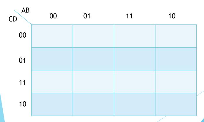
A Karnaugh map in constructed (in its most common form) for 4 variables in such a way that the combinations are ordered in Gray code order - starting from top left corner and in "zig-zag formation"
