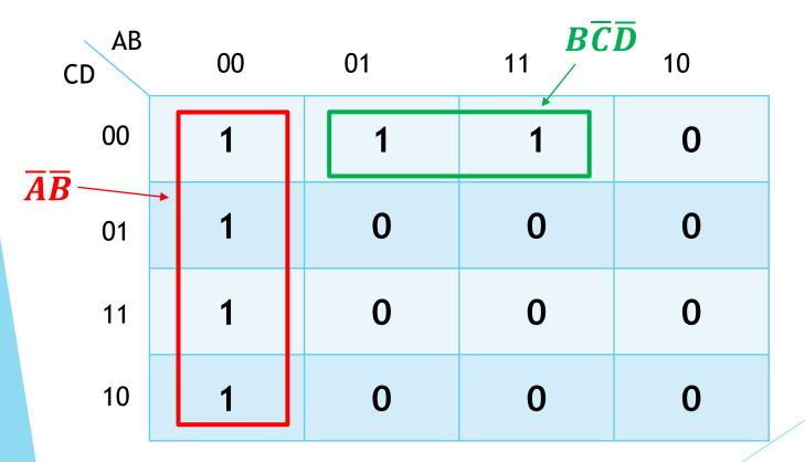
$$F = \overline{A}\overline{B} + B\overline{C}\overline{D}$$
