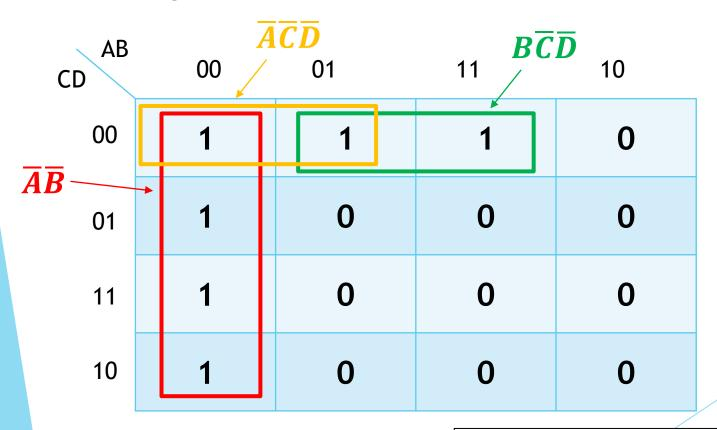
$$F = \overline{A}\overline{B} + B\overline{C}\overline{D} + \overline{A}\overline{C}\overline{D}$$
