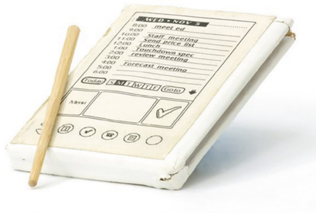
Figure 12.1 The PalmPilot wooden prototype
