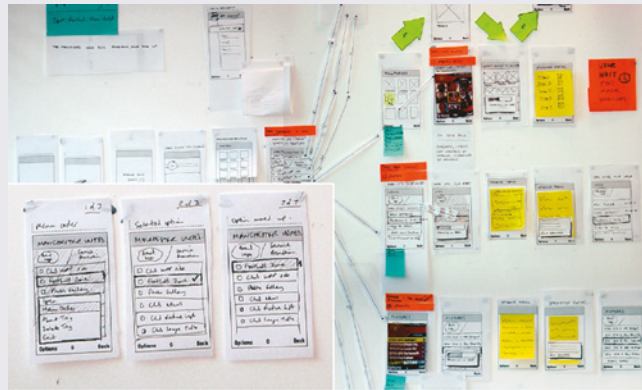
Figure 12.7 Prototype developed for cell phone user interface
