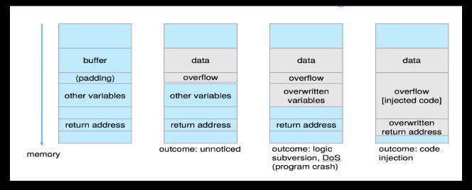
Frequently use trampoline to code execution to exploit buffer overflow:
