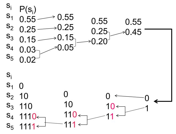
The probabilities affect the representation of each symbol in bits = bit patterns change according to the probabilities.
