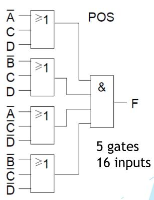
$$F = (\overline{A} + C + D)(\overline{B} + C + D)(\overline{A} + \overline{C} + \overline{D})(\overline{B} + \overline{C} + \overline{D}) \text{ (POS)}$$
