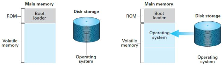
Step 1: Machine starts by executing the boot loader program already in memory. Operating system is stored in mass storage.
