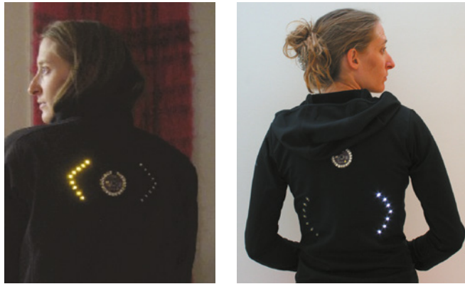
Figure 1.4 Turn signal biking jacket using e-textiles developed by Leah Beuchley
